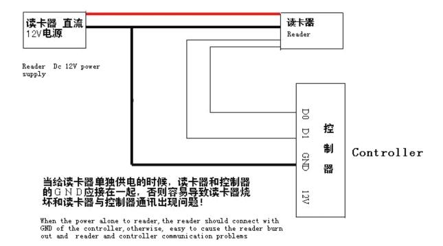
**1.3** Controller communication line (including 485/422, 232 and beat or other communication lines) suggest adopts internationally 8 core shielding twisted-pair cable, which can effectively prevent and shielding interference. Line diameter greater than 0.3 mm bus no more than 1,200 suggested length in 1000 meters of less than, if longer please choose other special 485/232 converter or add Repeaters, and choose the more thick communication cable.
