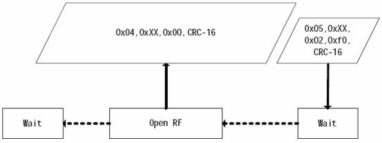
Notes: arrowed broken line stands for reader's inner flow; arrowed real line stands for the communication between reader and Epigyny computer.
