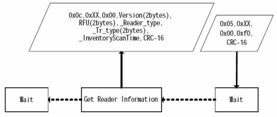
Notes: arrowed broken line stands for reader's inner flow; arrowed real line stands for the communication between reader and epigyny computer.
