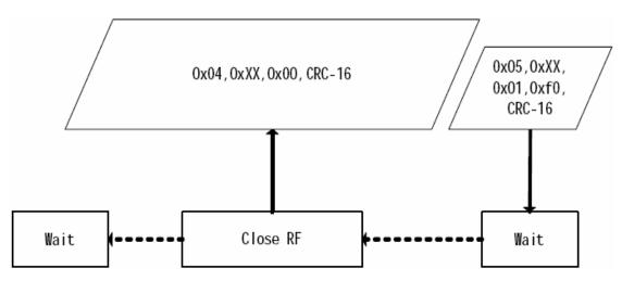
Notes: arrowed broken line stands for reader's inner flow; arrowed real line stands for the communication between reader and Epigyny computer.
